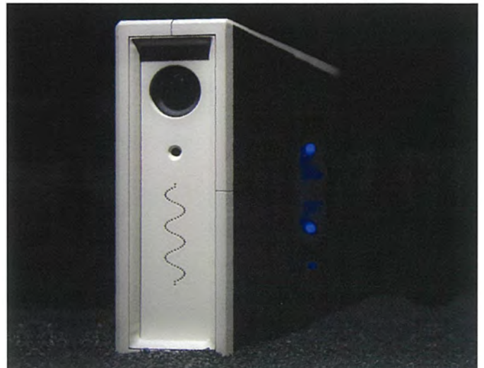
Input (camera) / Output – (projector) + Vent Detail for Speakers / Cooling
