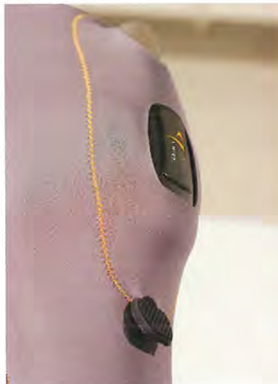
Arm unit containing CO2 inflation canister, trigger mechanism, GPS and electronics
